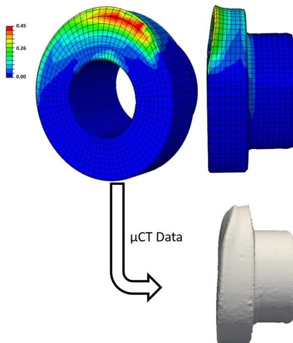
Figure 2: Plastic strain distribution on the lateral humeral bushing compared to  $\mu$ CT data from experimental tests
