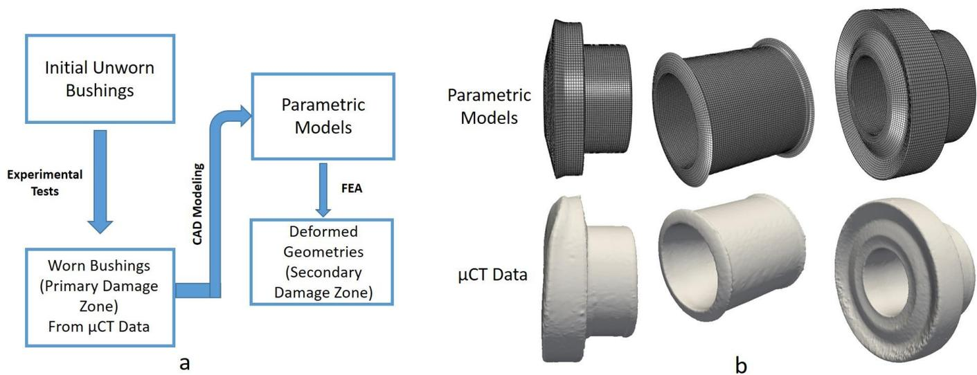
Figure 1: a) Parametric modelling procedure in order to analyze bushing damage progression b) Parametric modeling of worn bushing geometries based on  $\mu$ CT data
